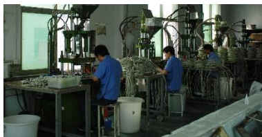
Vertical cables molding injection machines
